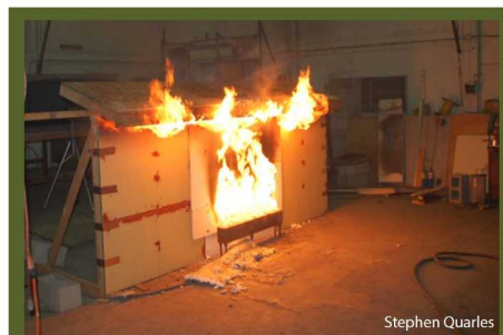
Flame impingement exposure to the underside of the eave, and time-to-ignition of the joists, blocking and fascia was quicker; and lateral flame spread faster, when an open-eave design was used in research experiments.
